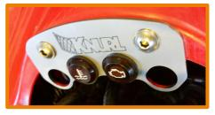
7. REINSTALL 2 END LIGHTS AND CHECK FULL RANGE OF STEERING. ENSURE NO CABLES RUB NEW DASH. ZIP TIE OUT OF THE WAY IF THIS IS THE CASE.
