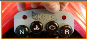
5. MOVE THE DASH TO THE SIDE AND ENSURE THERE IS NOTHING BELOW THE MARKED HOLES THAT WOULD BE UNINTENTIONALLY DRILLED THROUGH AND DRILL 1/4" HOLES WHERE MARKED.
